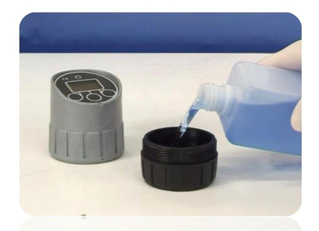
Add Reagent A to the top line (note; for lowest range test, volume is increased – use syringe)
